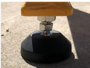
Adjust feet so the balancer is roughly level and tighten lock nuts on feet.
