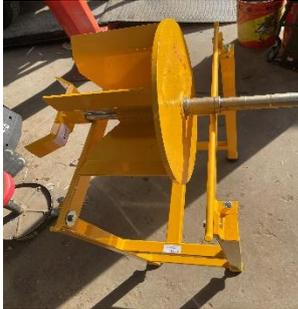
Allow the fan to roll by itself from one end to the other until it comes to a stop by itself, mark the top of the fan disc.
