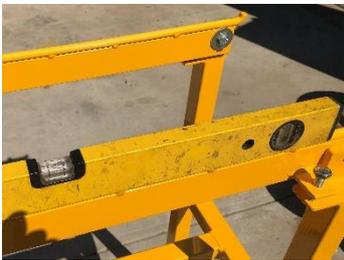
Place the spirit level along both runners (one at a time) and make level
