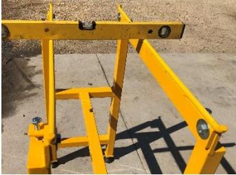
Place spirit level across two runners and adjust side bolts to make level
