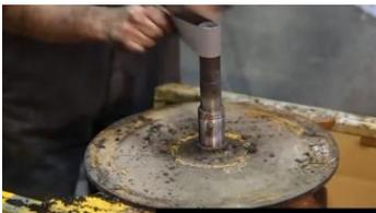
Clean up fan with hammer, grinder, or air chisel to remove all sugar and mog.
